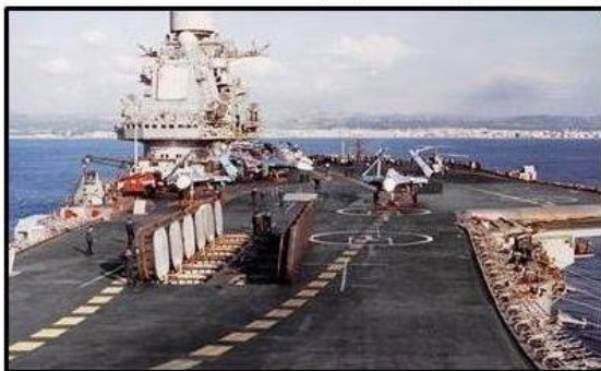
Air craft carrier Admiral Kuznetsov Clearly visible are the 12 launch pads for the GRANIT anti- ship missiles (Right) Photo's Euromaidan.com
